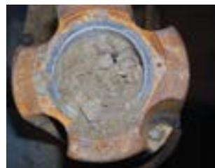
**Diaphragm Cavity Full of Mud Motor Shown Above**
