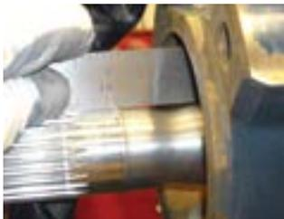
**Motor Shaft Damaged by Gravel in the Pump Intake**
