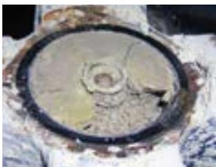
**Example of Diaphragm Cavity When Motor is Buried**
