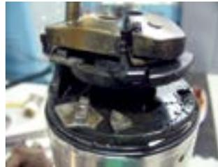
Extreme Shock Required to Fracture/Split Bearings
