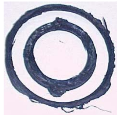
Figure 5: Destroyed upthrust washer
