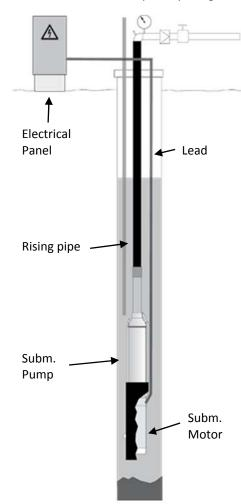
On the left, you will find a simple schematic of a typical borehole installation. From this, it is easy to deduct the challenges in selecting/sizing the right cable. Ideally, a cable that feeds a submersible borehole pump must:
