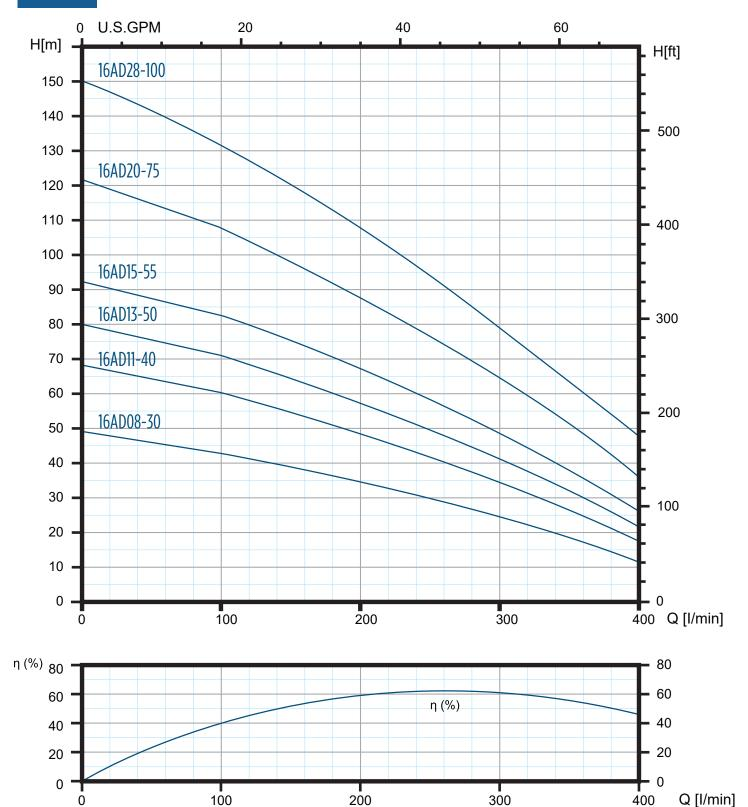
The hydraulic characteristics are guaranteed, according to ISO standard 9906:2012, grade 3B  $\,$
