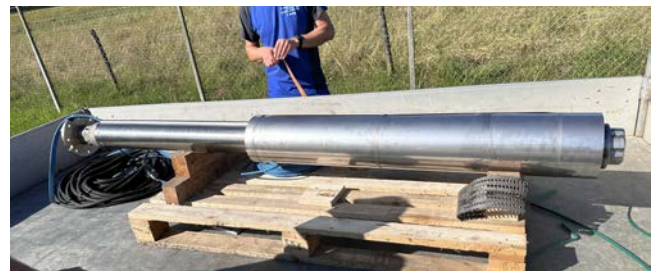
The Franklin Electric service team installed a 6-inch permanent magnet motor, submersible pump, cooling jacket, Variable Frequency Drive and PT100 sensor.
